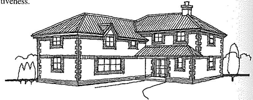
The excessive use of contrasting brickwork can be overfussy and unnecessary.
