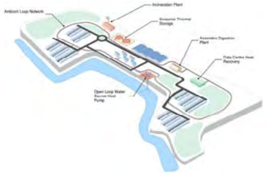
Fig 42 5G Ambient Loop District Heat Network
