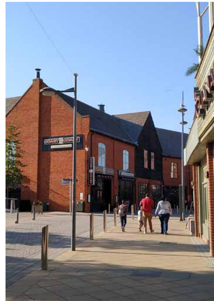
Figure 84: Example of lighting columns set at heights and positions to provide light to both pedestrian areas and the carriageway. It is recommended that LED lighting is used due to higher energy efficiency and power cost savings.
