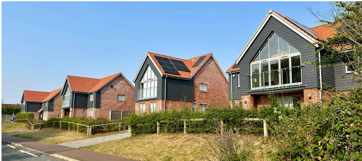
The setback from the street, and topography, create privacy for residents in these homes, despite the large glazing in Reedham.
