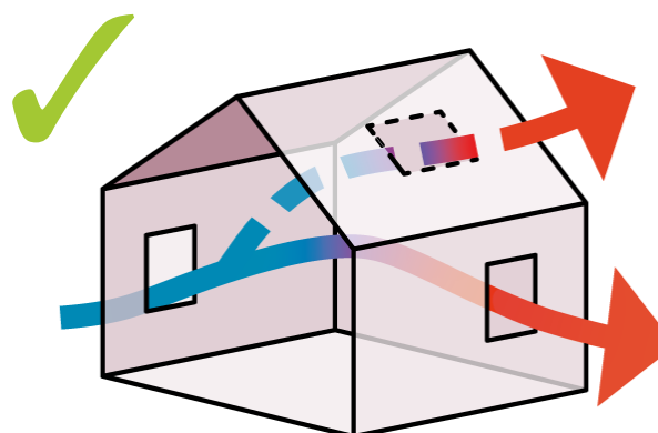
CROSS- AND STACK VENTILATION
