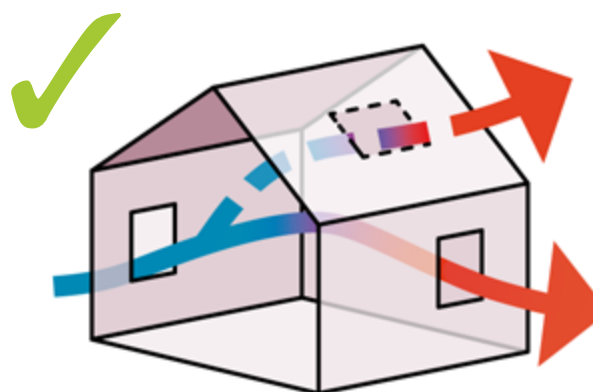
CROSS- AND STACK VENTILATION
