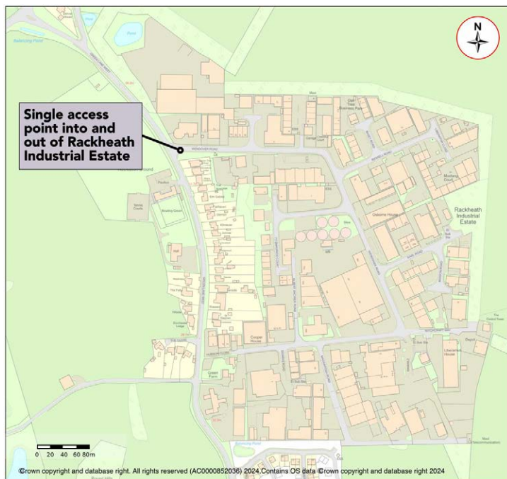
Figure 31: Single access point into and out of Rackheath Industrial Estate (source: Parish Online with own annotations).
