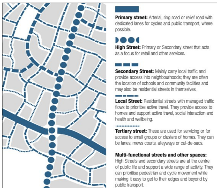
Figure 42: Street hierarchy: a typical neighbourhood street hierarchy. Source: National Model Design Code, part 2, page 9.
