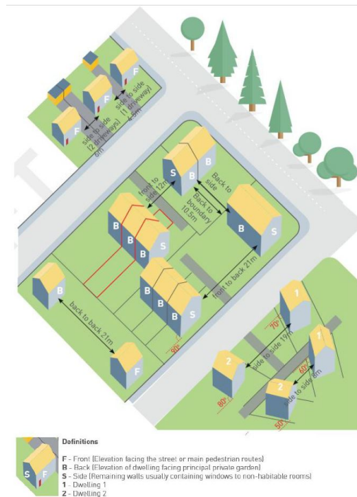
Diagram showing garden sizes and distances between houses (amended diagram from the North Norfolk Design Guide).
