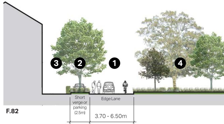
Figure 82: Cross-section to illustrate guidelines for edge lanes.
