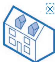
Loft conversion incorporating gable dormers which are out of scale and do not consider existing window rhythm or frequency,
