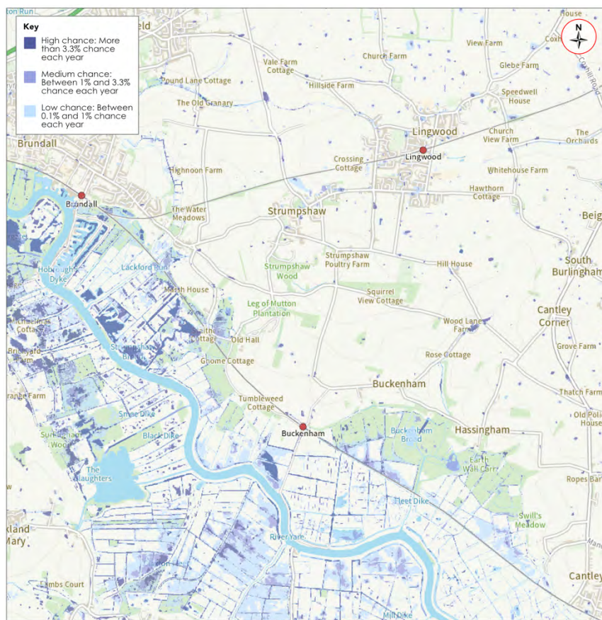
Figure 44: Surface water map (source: https://check-long-term-flood-risk.service.gov.uk/map , with own annotations). Blue line denotes parish boundary.
