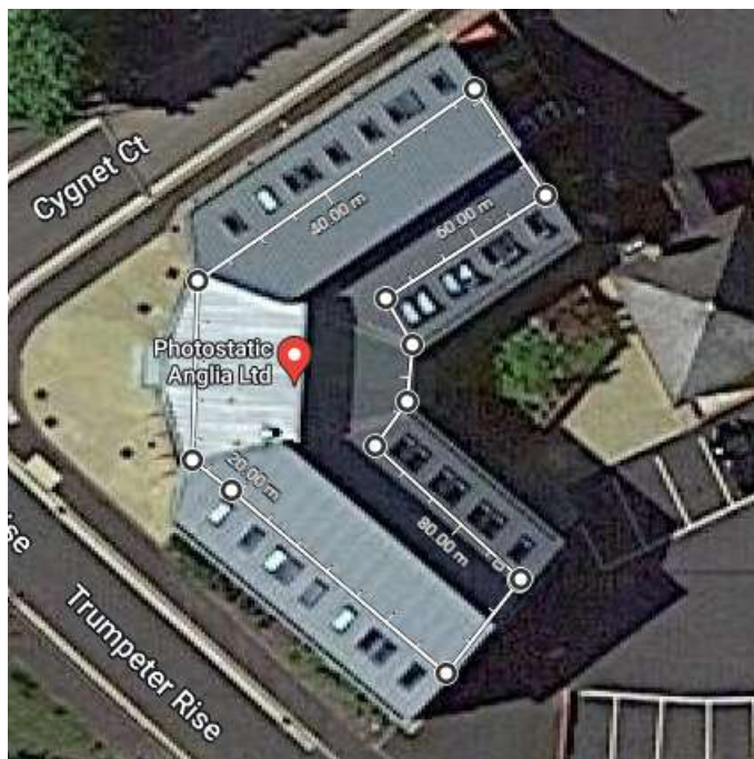
Figure 4: Potential Roof Space for Solar Arrays offering Day-long Generation Potential
